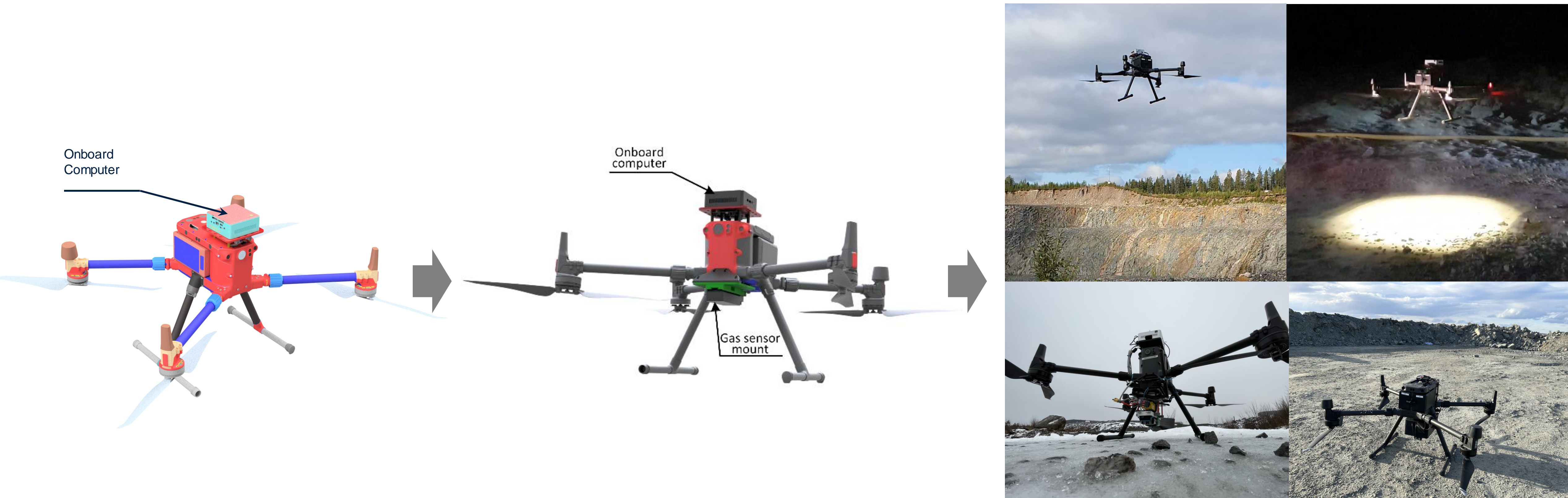
Figure 6. From CAD design of LTU-NUC aerial system to evaluation tests at Aitik
