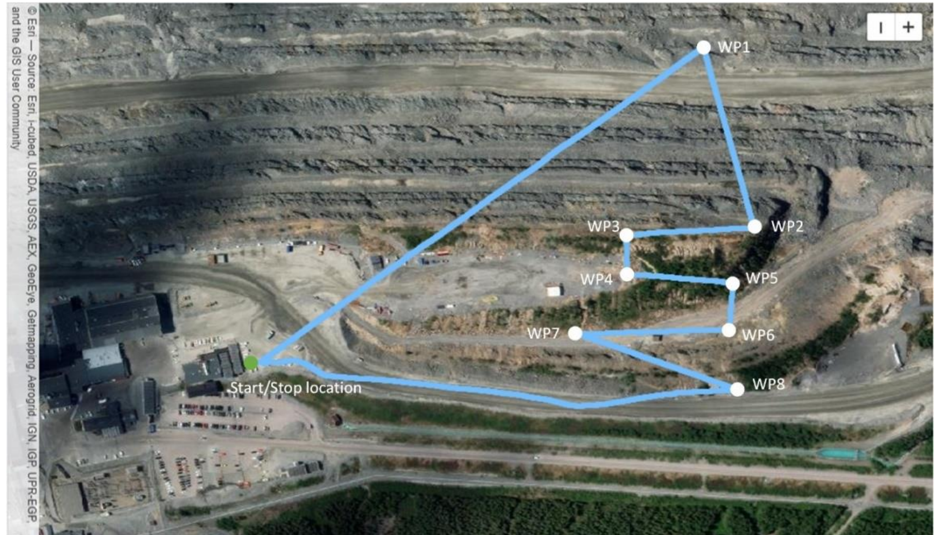
Figure 10. Full-scale mission flight path with assigned WPs for gas measurements.
