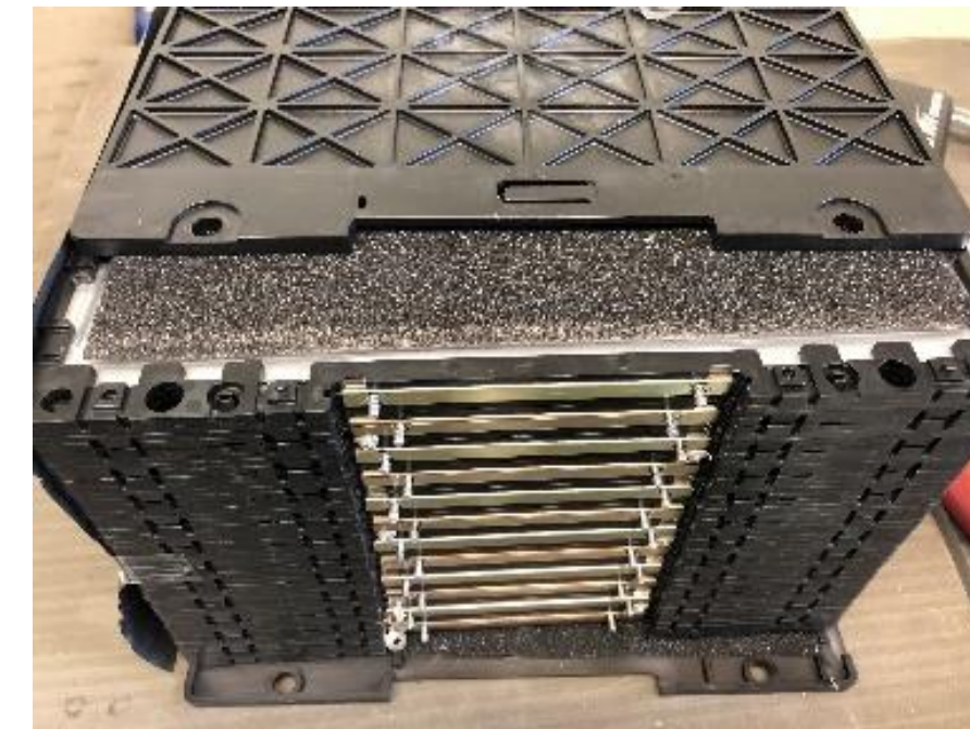
Dismantling the module down to cell level
