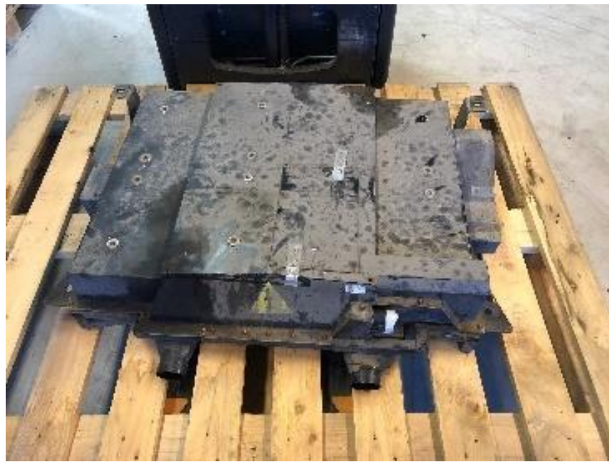
Flat battery pack before dismantling (Volvo C30; 150kg)
